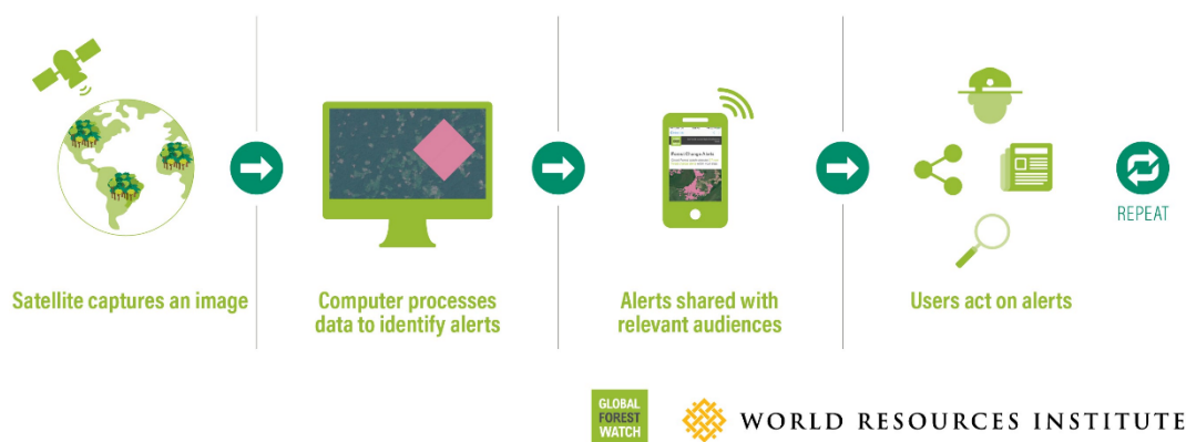
Figure 1: How Satellite-Based Deforestation Alerts Work: typical workflow from satellite imagery to action on the ground.
